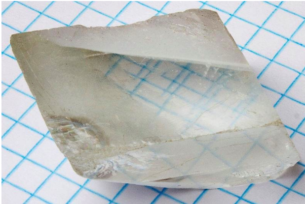
Calcite crystal on graph paper showing double refraction. The crystal splits a light ray into two rays causing 'double vision.'
