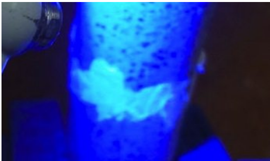
The repair to this vase can be seen under blacklight
