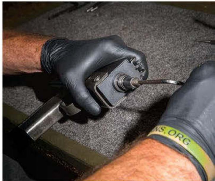
ISS is not only a full-service prop warehouse, it's also a licensed firearms manufacturer that employs numerous full-time gunsmiths and machinists. Here, one of its talented staff inserts a proprietary BFA (Blank Firing Adapter). The staff can tune the BFAs and blank cartridges to give the exact effect a director wants for the film. ISS' BFAs are so good, ISS provides them for several high-end customers, including NSWC Crane.
