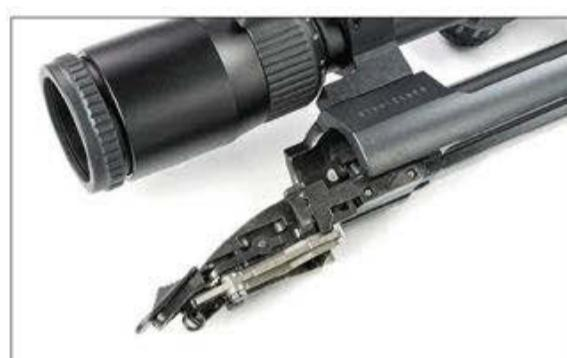
The bulk of the trigger components attach to the bottom of the receiver but are not enclosed.
