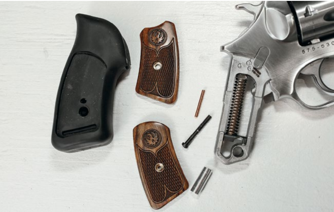
▣ The SP101’s hardwood panels are set into a rubber mono-grip that fits over the frame and is secured by a cross pin. The copper pin is for capturing the mainspring spring during disassembly.
