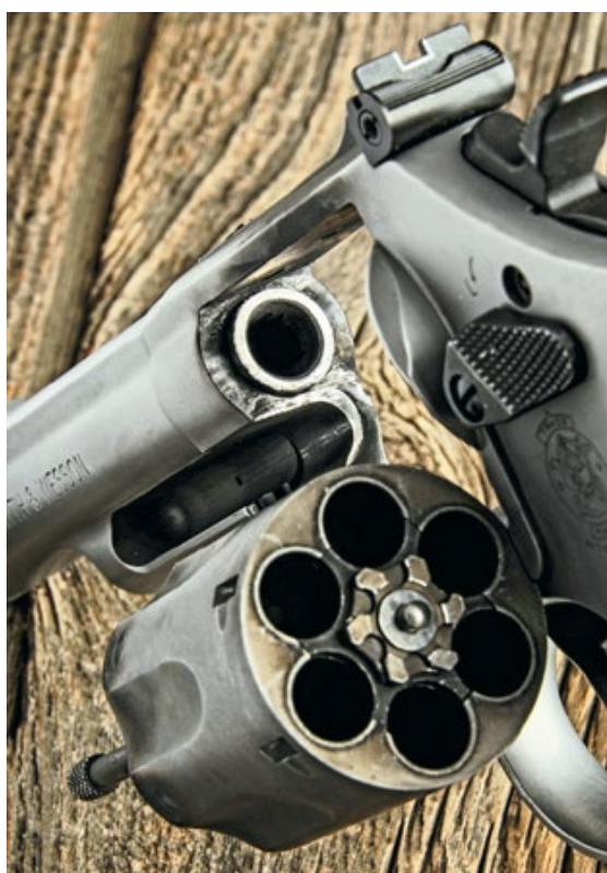
▲ The new K-frame magnums are more robust in critical areas, which prevents the distress cracking seen in older K frames that had been fed a lot of magnum ammo—as the author did during his test, with no problems.
