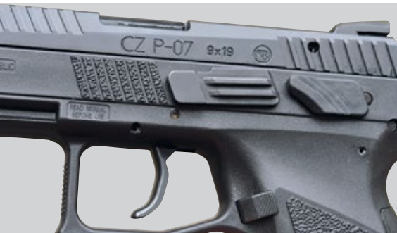
▲ The pistol ships with a decocker installed, with the option of changing to a manual safety, which is included in the box. The author dislikes this particular safety and recommends keeping the decocker.
