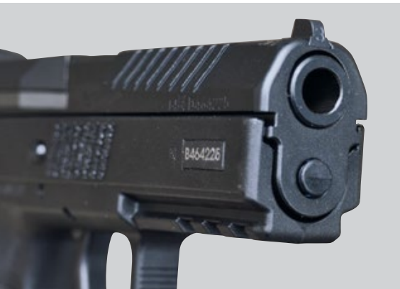
▲ The slide is relatively minimalist, so CZ has added front grasping grooves for ease of operation. The bore axis is very low, which results in a controllable gun with little muzzle rise.
