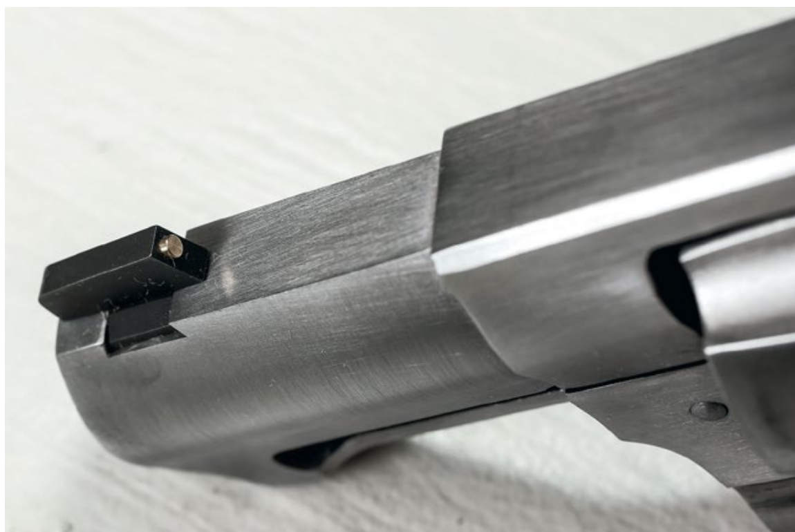
▲ The front is also a Novak and is also fit into a dovetail. It features a brass bead for good visibility even in low light.
