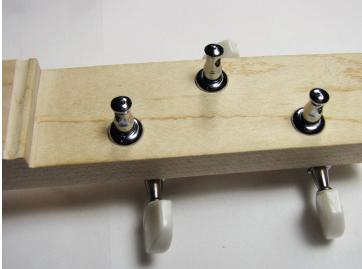
Try to leave at least 1 1/2" in between the tuners, so their buttons don't touch and any mounting plates they have don't get in the way of each other. The photo on the right shows a sample installation. Don't place the tuners too close to the edge of the recessed headstock area.
